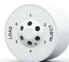
6 Port 2-position valve (1/16", SST, 400 bar, 0.3 mm) without valve drive (AVC26BC)
