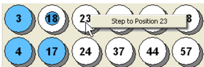
Fig. 64 Fraction Rack, Changing the Fraction Collector Position
