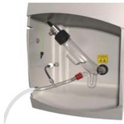
*Figure 32. Disconnecting fluids inlets*
