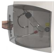
*Figure 31. Front window removal*
