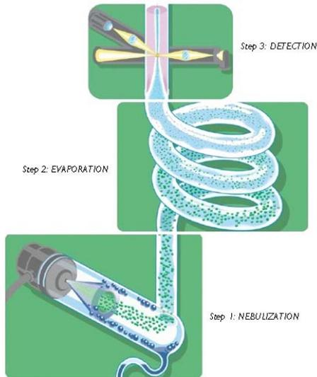
Figure 2. Cross-sectional View of the Detector
