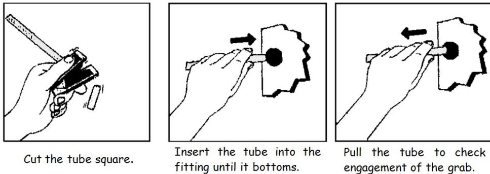
Figure 7. Inserting the Gas inlet tube
