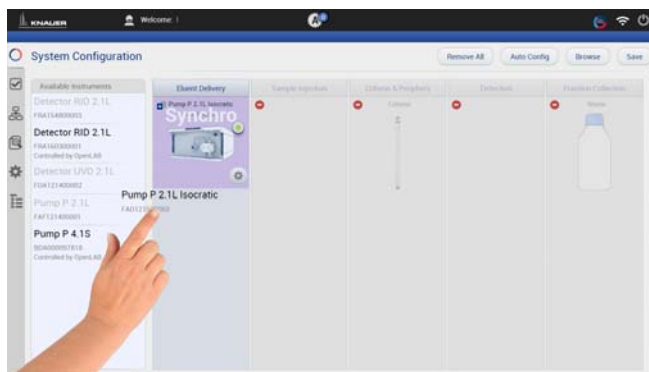
Fig. 5-14 Drag and drop second pump
